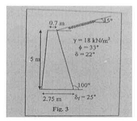
3. For an Anchored bulkhead system shown in figure determine the Anchor pull using free earth support method.
